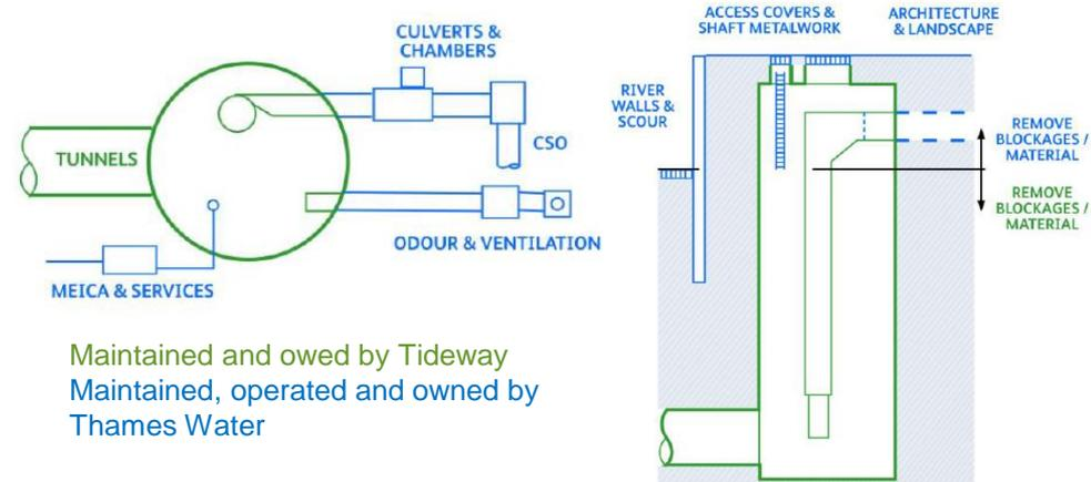
In the operational phase Tideway's only business is the maintenance of a gravity operated tunnel
