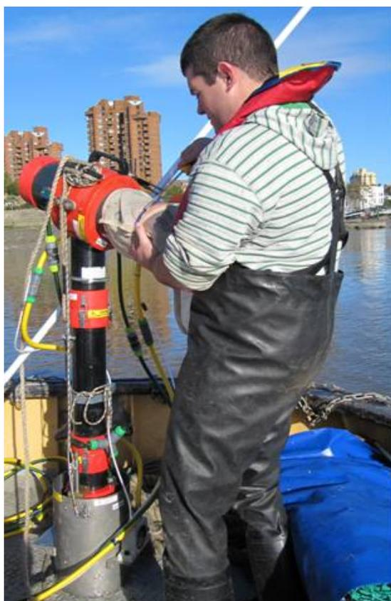
**Vol 3 Plate C.43 Airlift sampler submerged into subtidal zone of the Thames**
