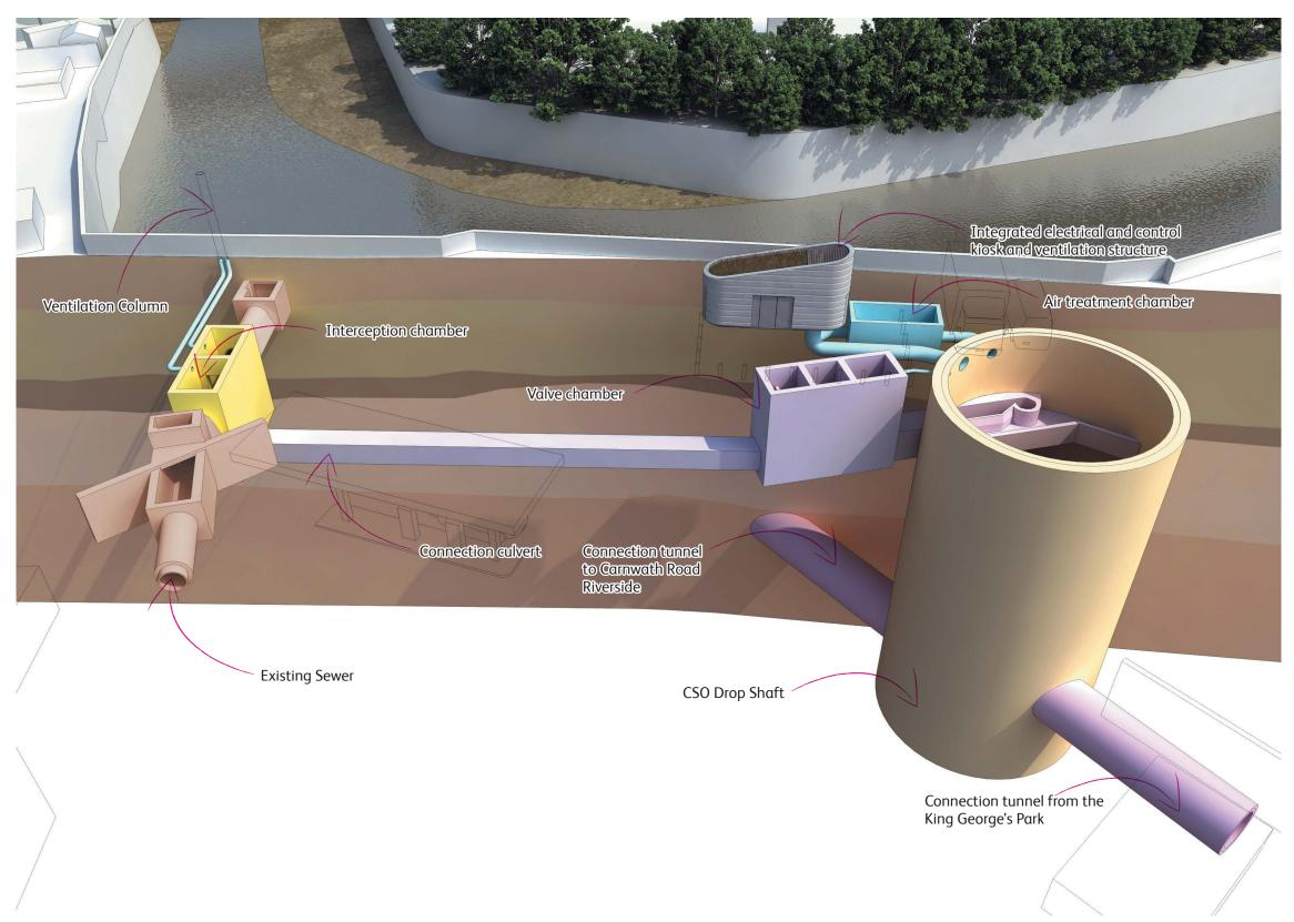
Figure 10.24: Proposed functional components diagram: below ground view
