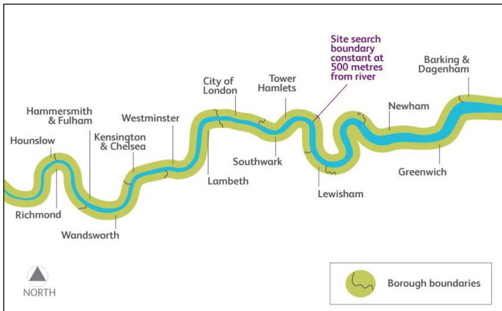
4.3.12 The approach to the search area for CSO sites was more localised than for the main tunnel sites. Each CSO was allocated an individual area of search, the extent of which varied depending on the sewer network upstream and downstream of the current overflow structure, and the river outfall/outlet location. However, all CSO sites needed to be as close to the existing line of the sewer as practicable and therefore the areas of search needed to include the river foreshore.
