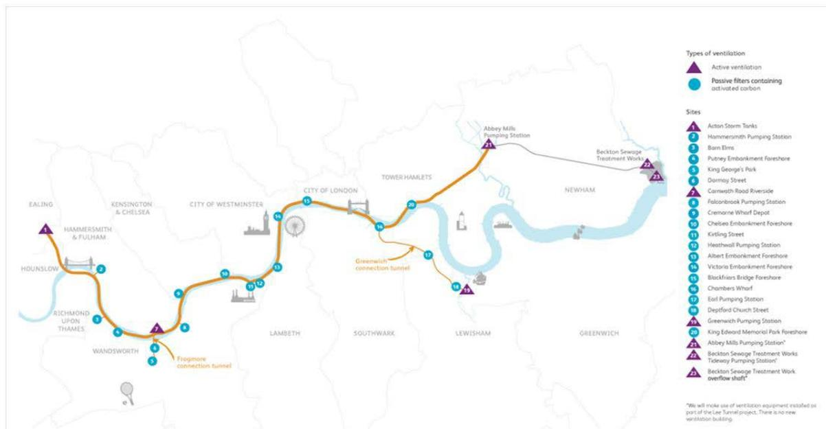
6.5.7 The *Air Management Plan* demonstrates how Thames Water would limit the extent of nuisance odours and significant loss of amenity as required by NPS paras. 4.3.11 and 4.3.14. This would be achieved by not exceeding 1.5 odour units per cubic metre as an hourly average concentration level for 98 per cent of the typical year at surrounding sensitive receptors.
