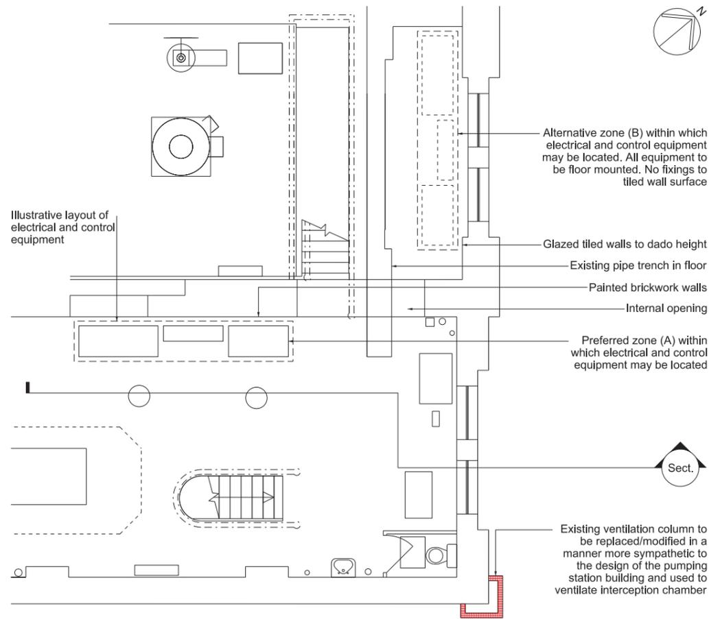
Intervention into pumping station (ground floor plan)
