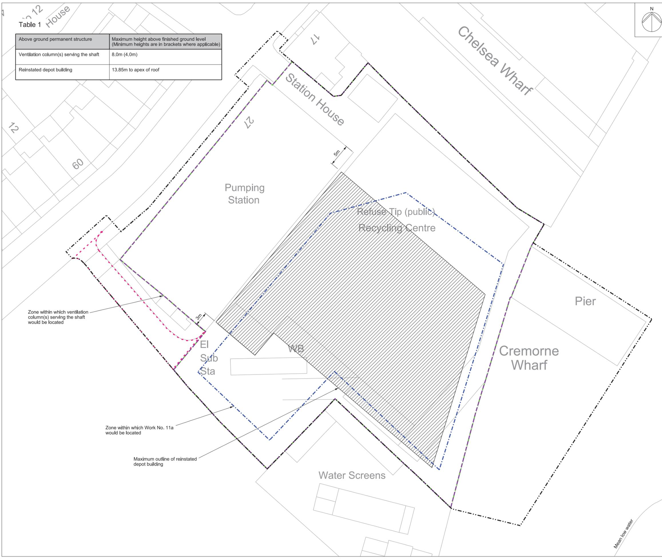
Zone within which ventilation column(s) serving the shaft would be located
