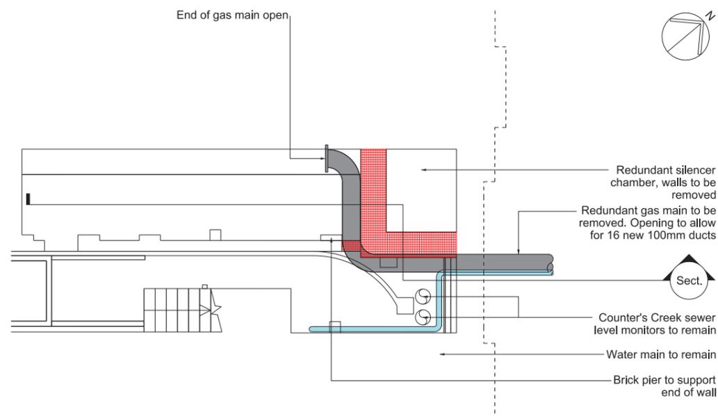
Intervention into pumping station (basement plan)
