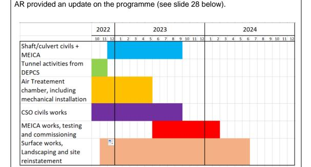
MEICA\* - Mechanical, Electrical, Instrumentation, Control & Automation features
