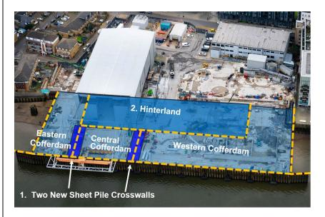
STAGE 1 – Installation of two sheet pile crosswalls
